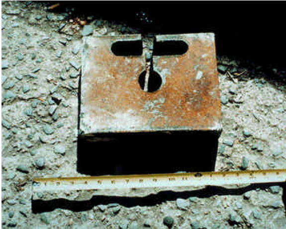
FIGURE 4.10 This is the metal counterweight which fell off the building and struck the man in the head.
